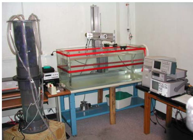
Figure 3.6 The computer controlled exposimetry system and electrical drive system for the 2 x 2 array utilized in measuring the spatial and temporal dependent power output of the array.
