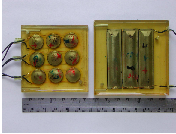
Figure 3.8: Size comparison of 3x3 circular and 3x1 rectangular cymbal transducer arrays
