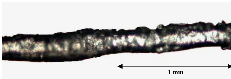
Figure 4-2. HC/PDMS (Dipped#1) Fiber (10X Magnification)
