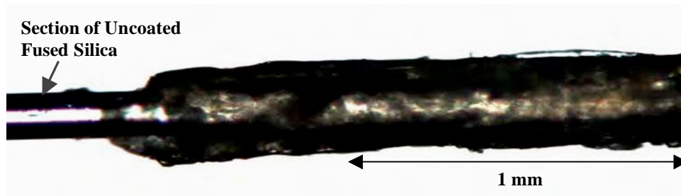
Figure 4-5. FPOL/PDMS (Applicator) Fiber (10X Magnification)
