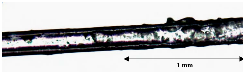
Figure 4-3. HC/PDMS (Dipped#2) Fiber (10X Magnification)
