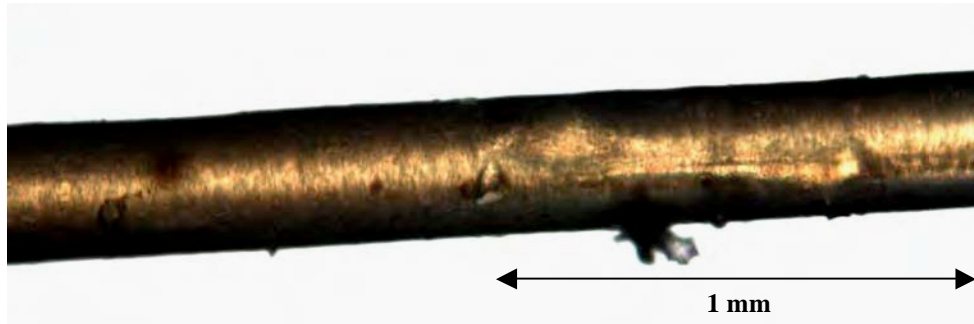
Figure 4-4. HC/PDMS (Applicator) Fiber (10X Magnification)
