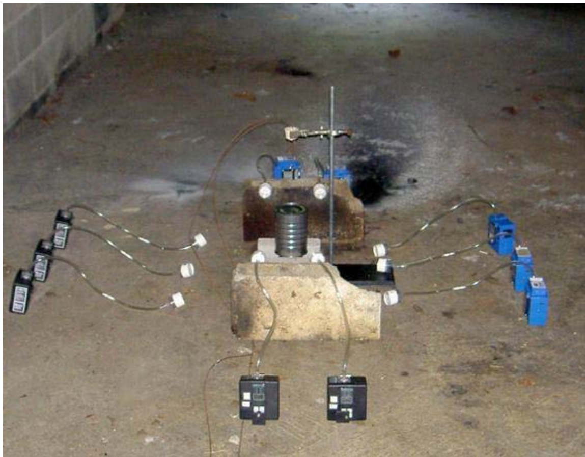
Figure 2-2. Placement of CS sampling trains inside of the mask confidence chamber.
