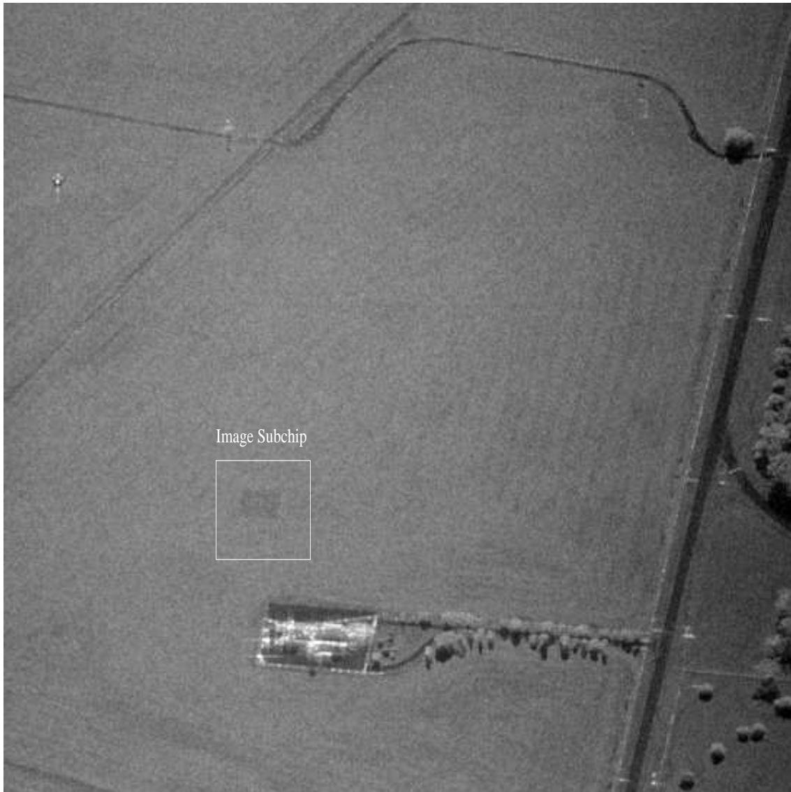
Figure 37: Intensity SAR image generated from the repeat pass collection processed to a 3 dB resolution of 0.61 m (range) by 0.15 m (azimuth) with a Hamming window applied. Also shown is the image subchip selected for further processing and change detection analysis.
