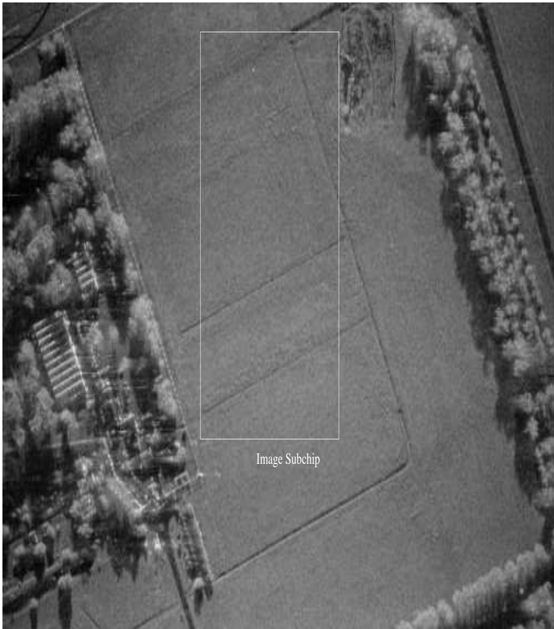
Figure 48: Intensity SAR image generated from the repeat pass imaging collection processed to a resolution of 0.52 m (range) by 0.150 m (azimuth) with a Hamming window applied.
