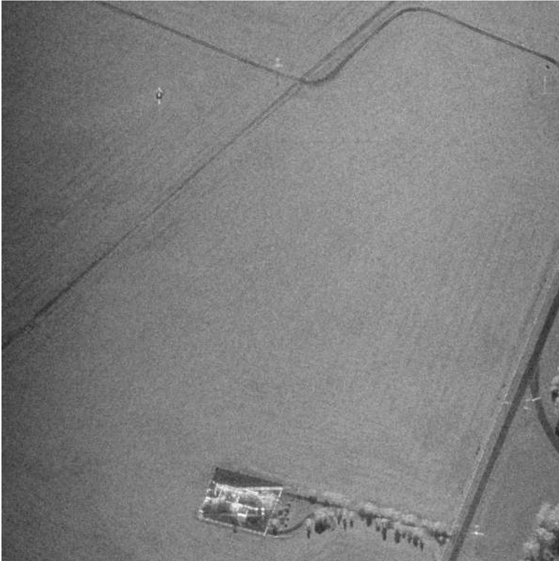
Figure 11: Primary collection intensity image. The image has been processed to a resolution of 0.58 m (range) by 0.150 m (azimuth) with a Hamming window applied.
