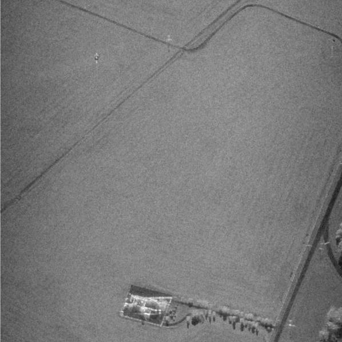
Figure 12: Repeat pass collection intensity image. The image has been processed to a resolution of 0.58 m (range) by 0.150 m (azimuth) with a Hamming window applied. The temporal baseline for the repeat pass interferometric pair is approximately 12 minutes.
