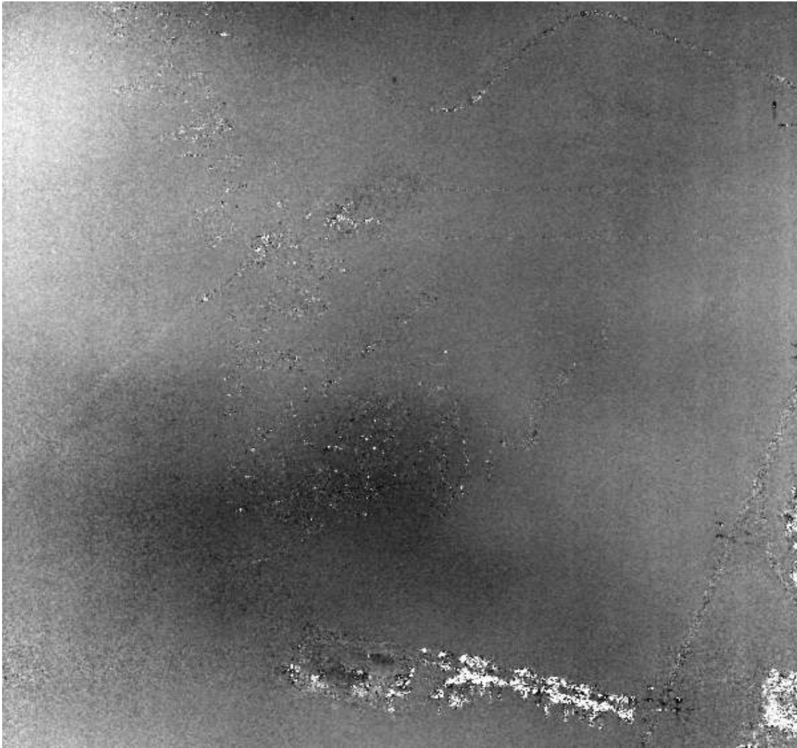
Figure 14: Phase image of the sample complex cross correlation coefficient obtained by spatially averaging over a sliding estimation window (2 by 6 pixels in range and azimuth respectively).
