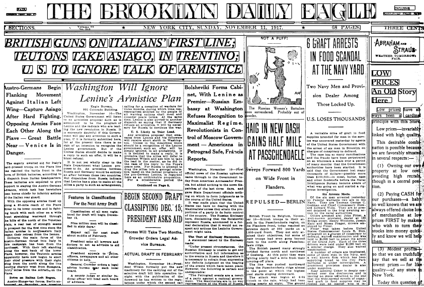
Figure 3: Automatic zone segmentation for the Brooklyn Eagle without first removing lines. Notice that many columns are merged.
