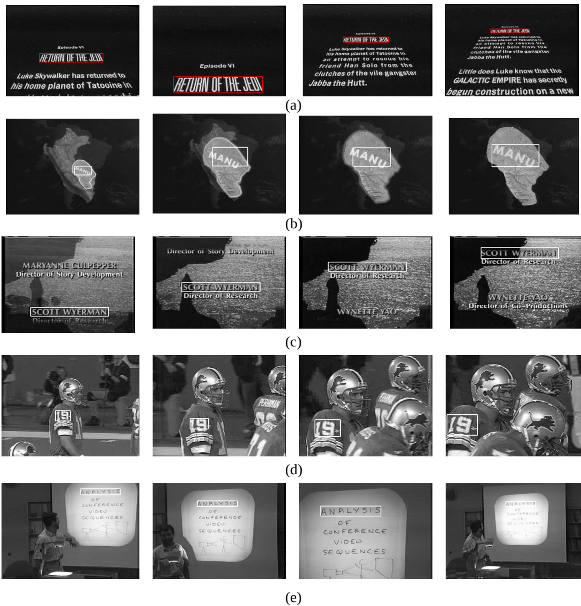
Figure 21: Demonstration of TextTracker 's performance on various video sources. The initial position of the text block is manually specified. (a) Tracking of movie credits: Text zooming with displacement. (b) Zooming scene text. (c) Text scrolling up across varying background. (d) Tracking text on a football athlete's jersey. (e) Tracking text in a conference room scene. All of these and other tracking results can be found as MPEG video at http://documents.cfar.umd.edu/LAMP/Media/Projects/TextTrack/
