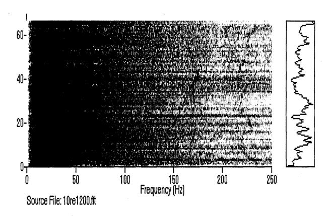
At ranges greater than 1000 feet, the engine harmonics are absorbed by the atmosphere.
