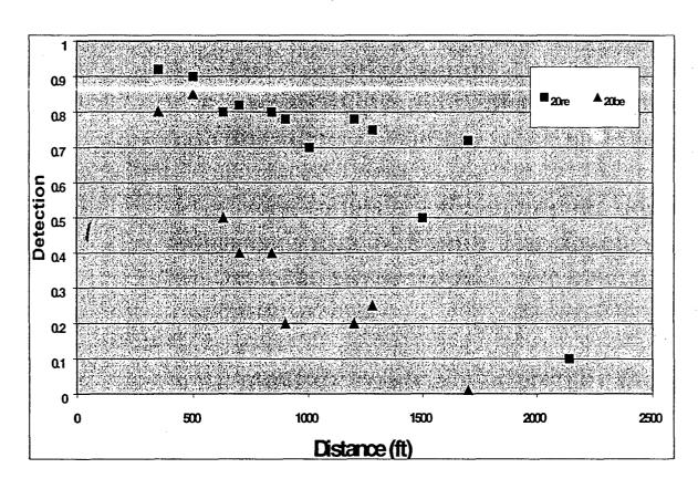
Detection versus range for regular track and band track at 20 mph with exhaust facing the array.
