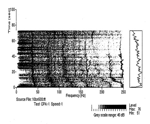
Band Track line structure at 40,80, and 120 Hz for 10 mph.
