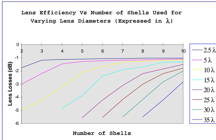
Figure 2 – Luneberg Lens Sizing/Efficiencies for Various Lens Thicknesses (expressed in wavelengths)
