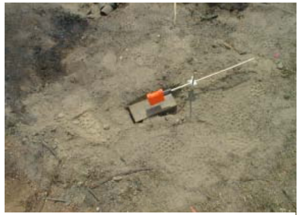
Figure 3: Small REMIC-II positioned over a PMD-6 AP Mine.
