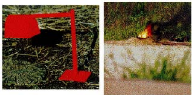
Figure 2: REMIC device on the left, and burning AT landmine following REMIC initiation.
