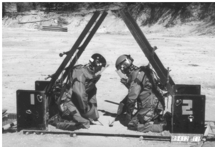
Figure 1 - Mannequins placed in kneeling position, dressed in HDE with Sport-1 helmet on mannequin 1 (left), HDH-1 helmet on mannequin 2; simulated mine 0.66 m from both sternums
