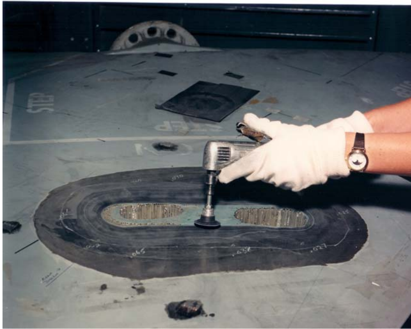
Figure 3: Formation of the scarf in the F/A-18 Horizontal Stabilator using a hand-held router
