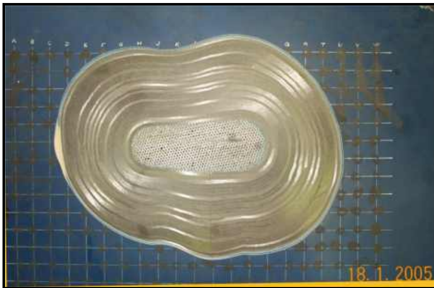
Figure 4: CNC Machined scarf cavity
