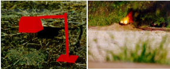
Fig 2: REMIC device (left) and burning mine (right)
