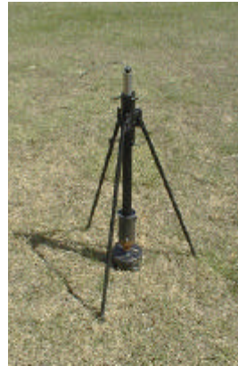
Fig 1: Bullet with Chemical Capsule (BCC)
