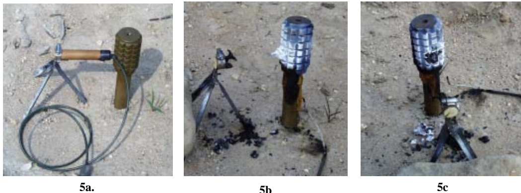
Figure 5a: Unfused live POMZ-2, flare positioned from stand at side of mine. 5b: POMZ-2 after flare burned, TNT melted and flowed at bottom. 5c: Burned POMZ-2 after slug removed.
