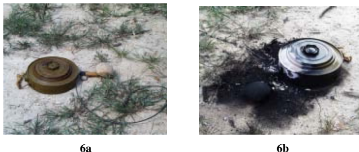
Figure 6a: TM-46 AT mine. Flare placed on the ground aimed at the side of the mine case. 6b: Mine after flare burned.
