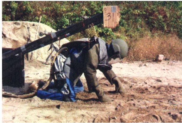
**Figure 1.** Mannequin placed in crouching position, illustrating versatility of mannequin positioning apparatus
