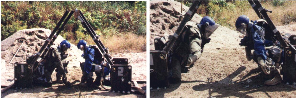
**Figure 2.** Mannequins kneeling on one knee, dressed in HDE with Sport helmets and positioned 0.66 m between sternum and simulated blast AP mine (200 gram C4); a) pre-blast (left), b) post blast (right)
