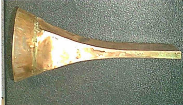
Figure 3.8: Acoustic Wave Guide
