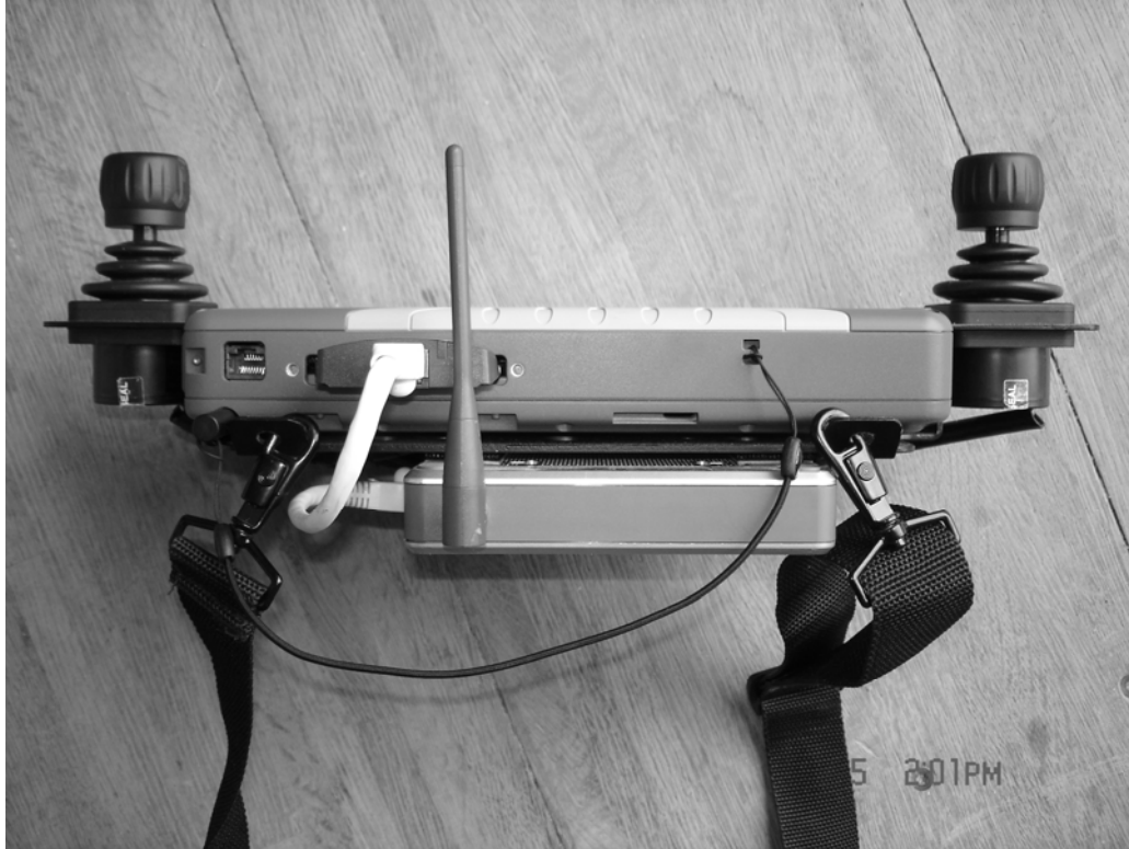
Figure 5. ARL OCU showing ad hoc node.
