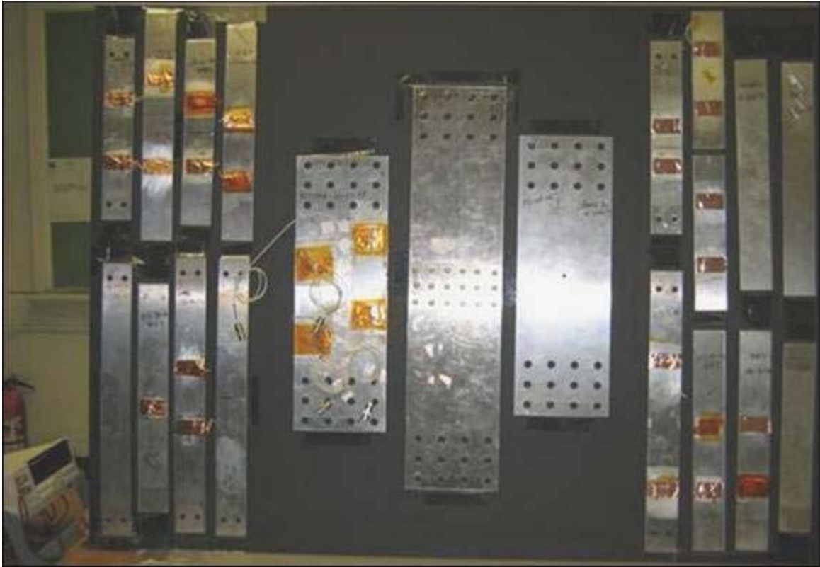
Figure 3. Part of the total number of specimens that were fabricated, precracked, and tested for developing the structural health monitoring technique.
