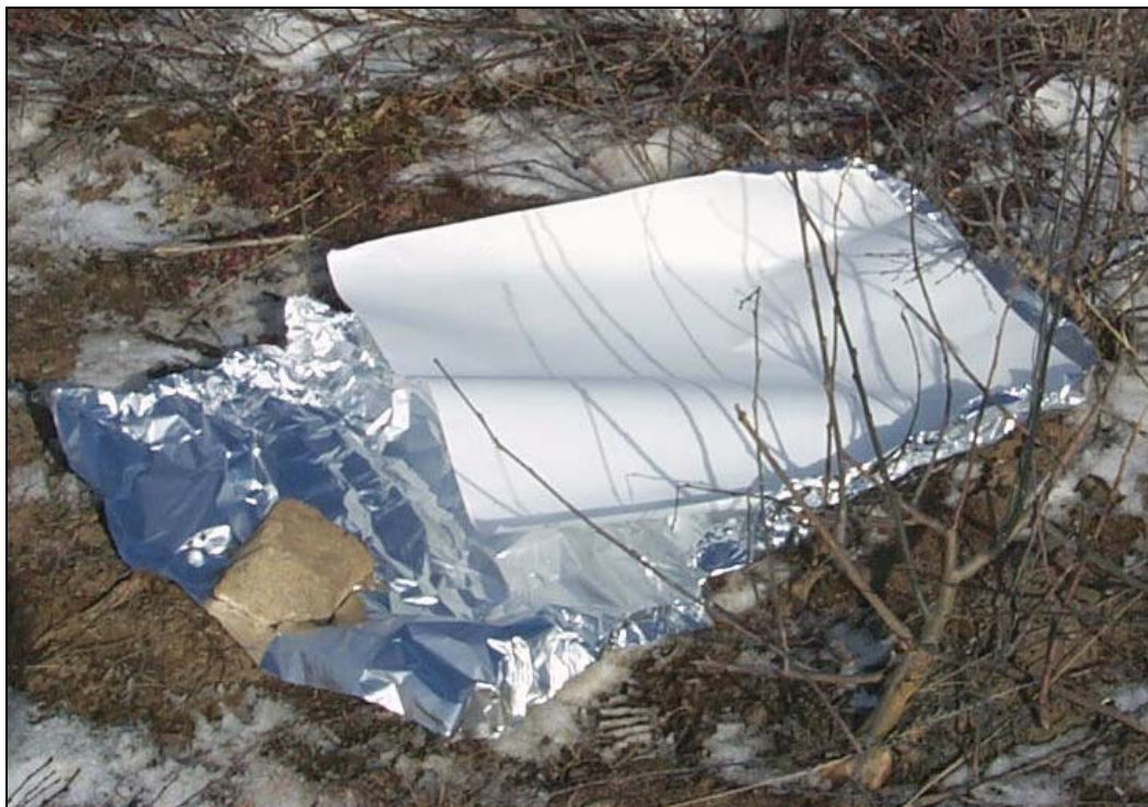
Figure 1. Filter papers (52 by 52 cm) on foil backing used for fogging event #1.
