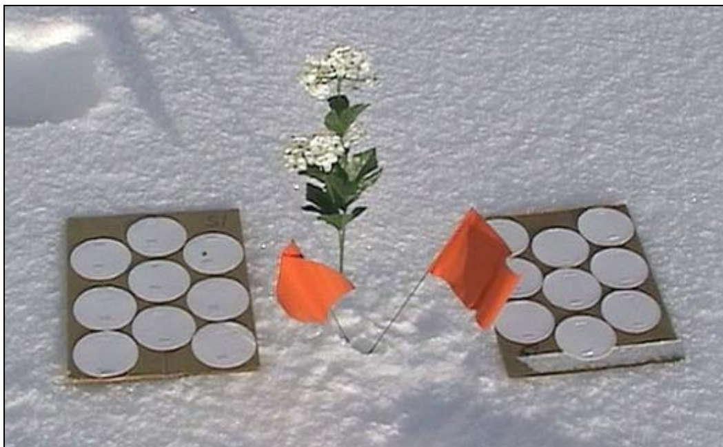
Figure 2. Arrays of nine 7-cm-diameter glass microfiber filters used for fogging events #2, #3, and #4. The arrays were used with synthetic vegetation, as shown above, in events #3 and #4.
