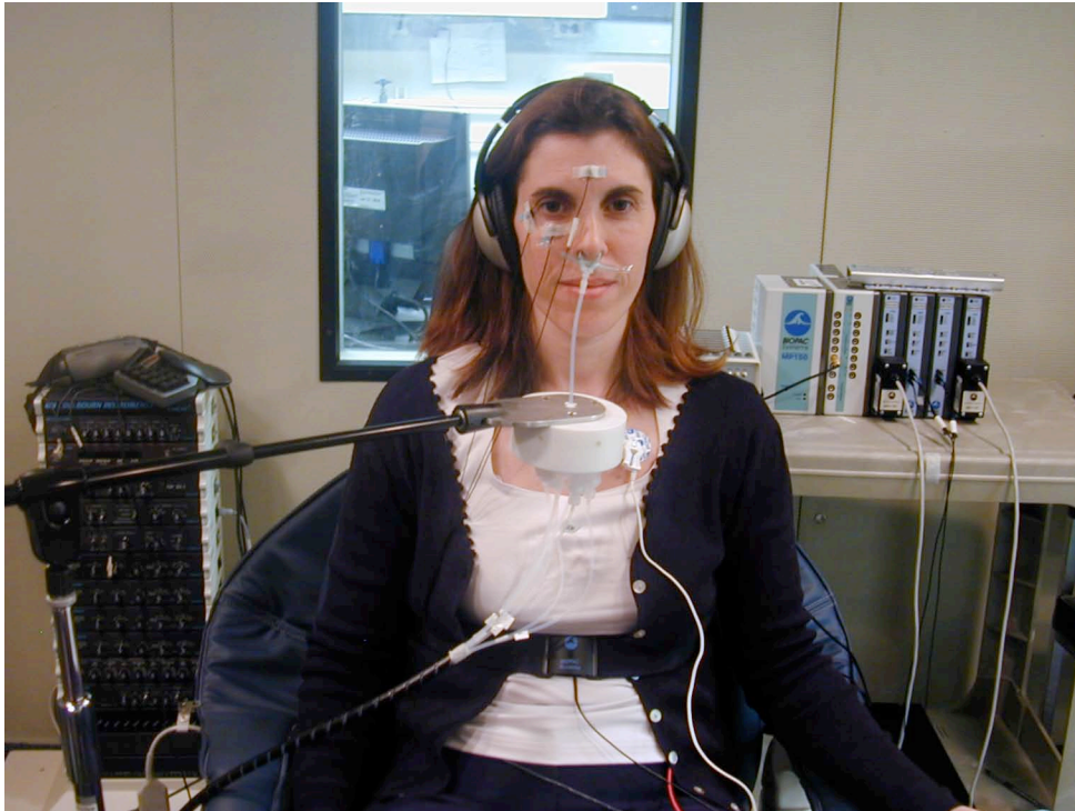
Fig. 8: Olfactometer manifold combined with an auditory startle experiment. The manifold containing the odors is placed close to the subjects nose to allow rapid and sharp delivery.
