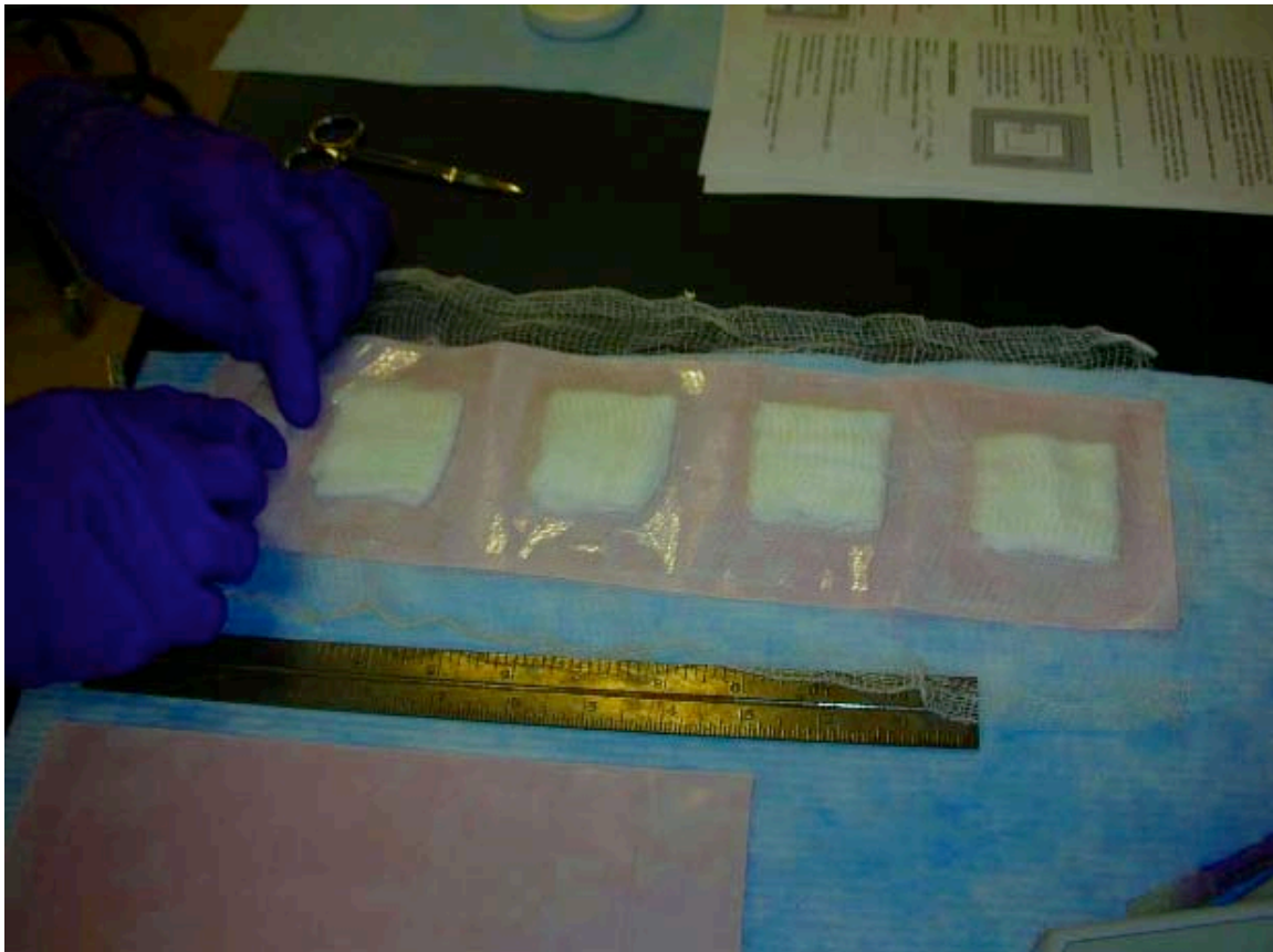
Figure 1: Because there is no commercially available product suitable for the sweat collection, we developed our own sweat pads that were optimized for both the physical rigors associated with the skydive, as well as the purity required for GC-MS.
