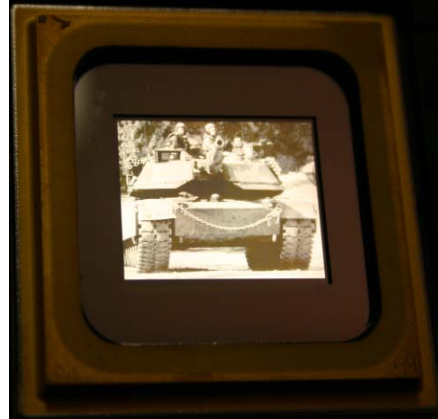
Figure 14: SXGA DMD Displaying an Image
