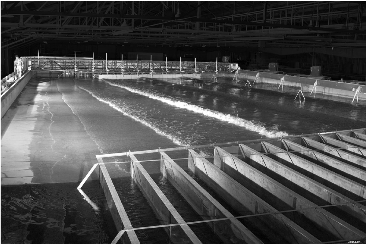
Fig. 1. Oblique view of the Large-scale Sediment Transport Facility (regular wave experiment). A technician standing in the upper left corner indicates the physical size of the facility.
