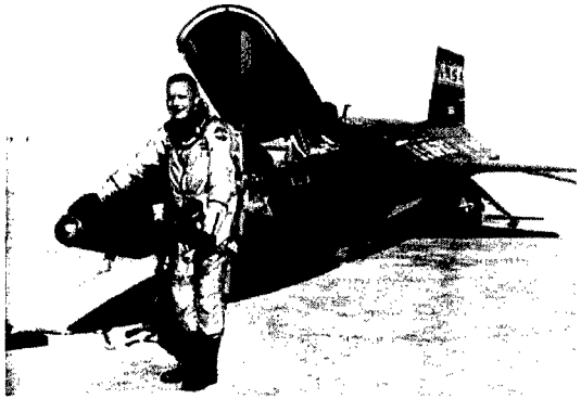
NASA research pilot Neil A. Armstrong following a 1960 X-15 flight. He is wearing a full pressure suit. This not only protected against depressurization, but also from heating and wind blast during a high-speed/high-altitude ejection. This eliminated the need for an escape capsule. NASA photo
