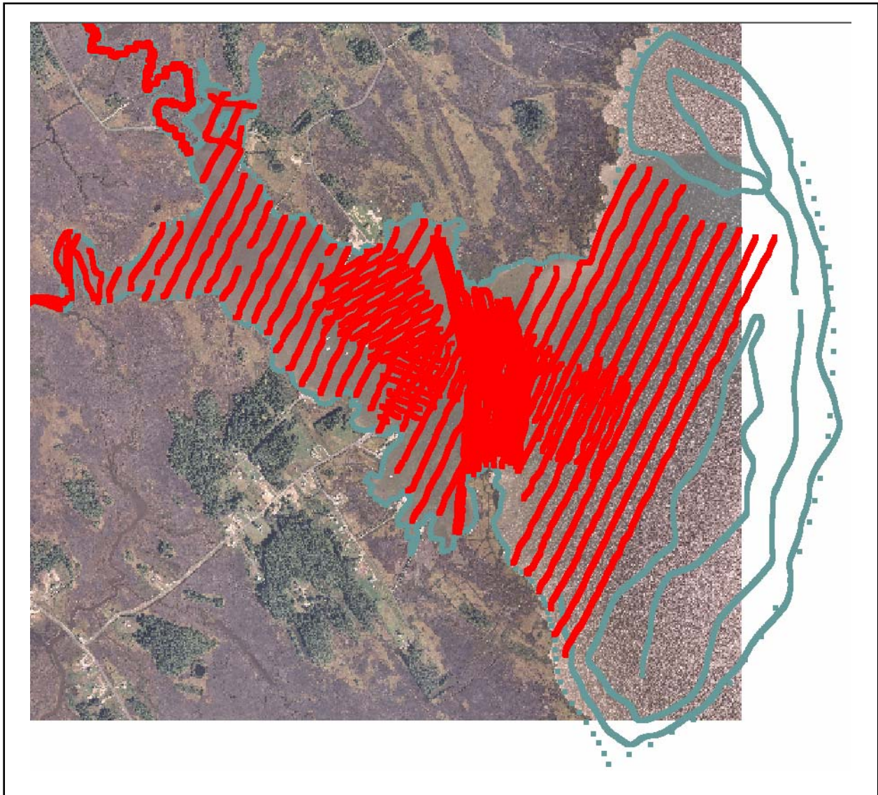
Figure 3. Scatter data points representing bathymetric survey locations for Tedious Creek
