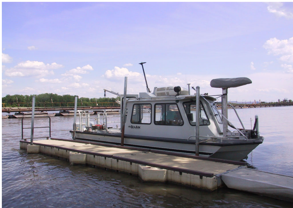
Figure 4. Data collection boat. Multibeam bottom profiling, ADCP velocity, and sediment data are all collected from this single platform. This boat is GPS equipped and fully compensated for pitch, heave, and roll
