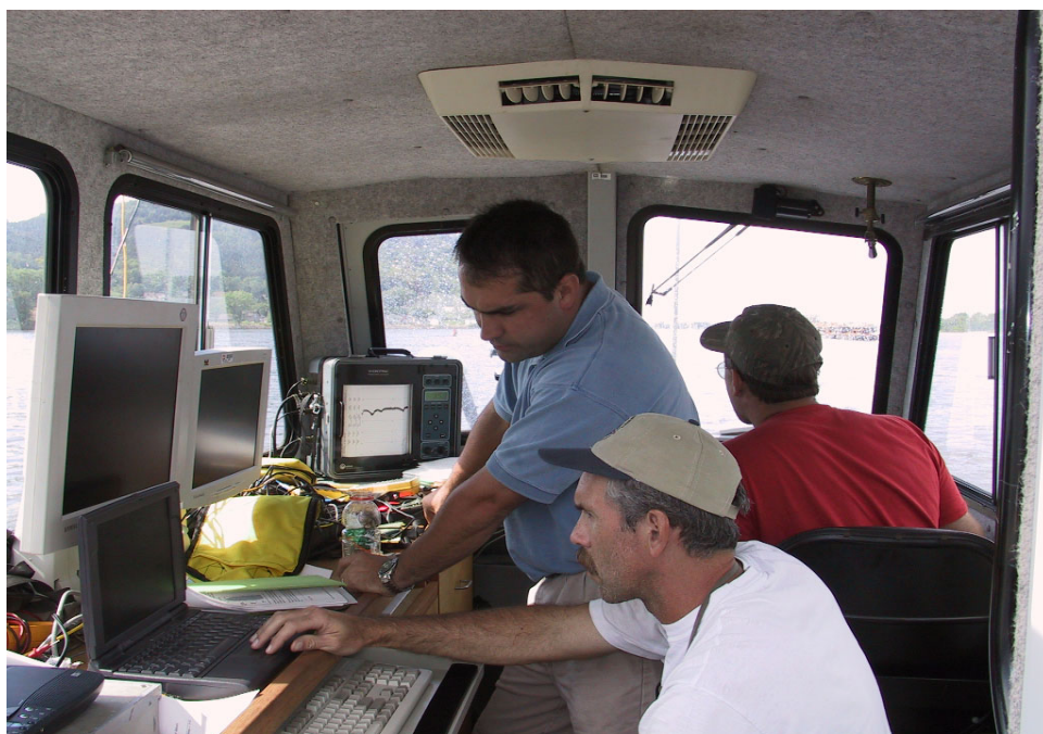
Figure 5. Onboard computers show boat location at any time and monitor all data collection activities. Boat position is monitored and used by multibeam and ADCP instruments and computers
