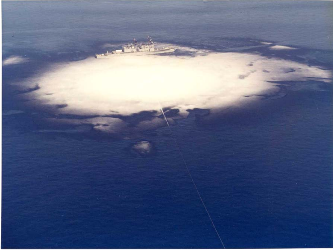
Figure 3. Photograph of Bulk Cavitation Due to UNDEX Event
