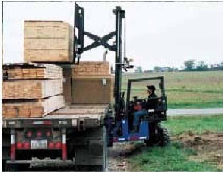
Figure 7: Illustration of the extendable reach capability required of the proposed forklift
