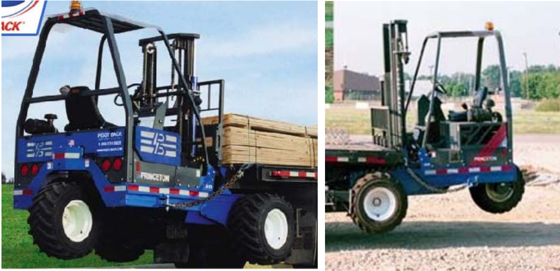
Figure 8: Demonstration of the truck transportable capability
