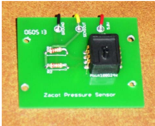
Figure 15. Honeywell Pressure Sensor/Transducer on a PCB Mount
