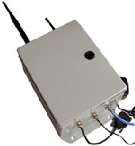
Figure 12. SPB400 Stargate in Hardened Case for Use in Shipboard Setting [Ref 7]
