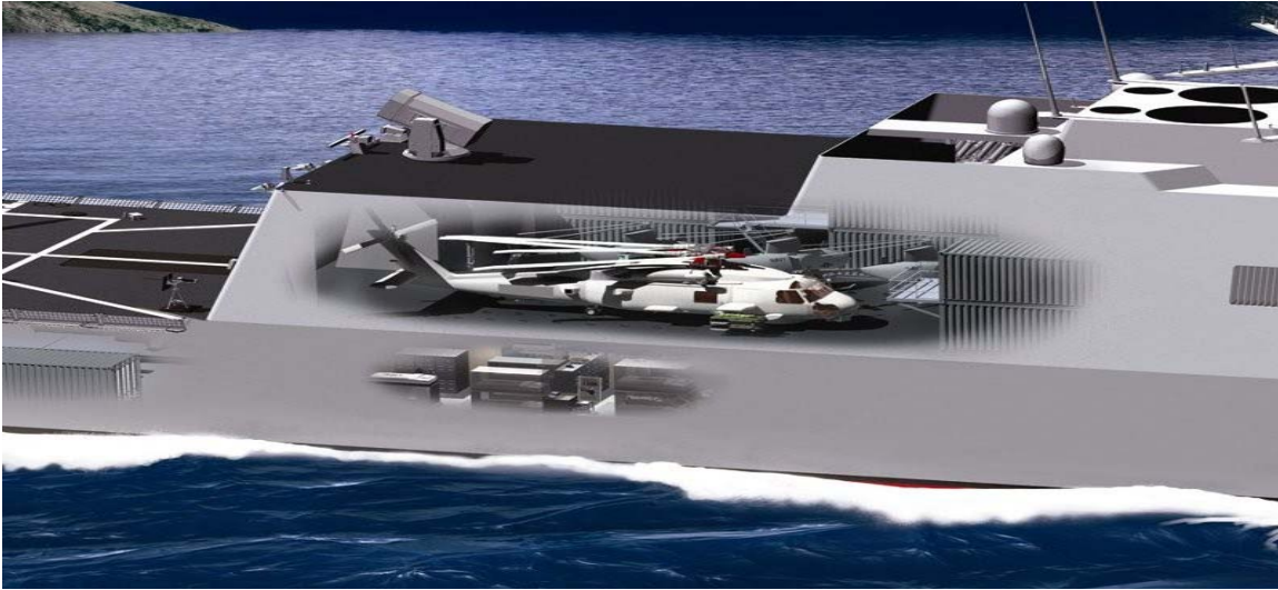
Figure 17. LM LCS Crew Areas, Aircraft Hangar, and Weapon Module Stations 75
