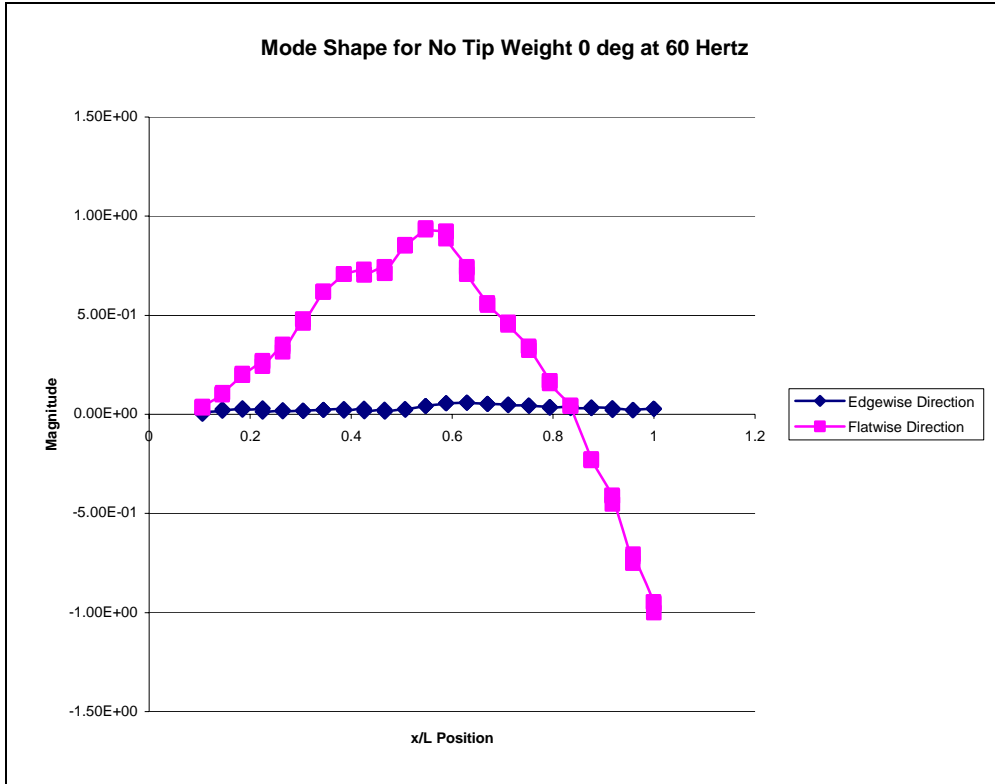
Figure 22: Mode Shape for No Tip Weight at Zero Degree Root Pitch Angle With a 60Hz Frequency
