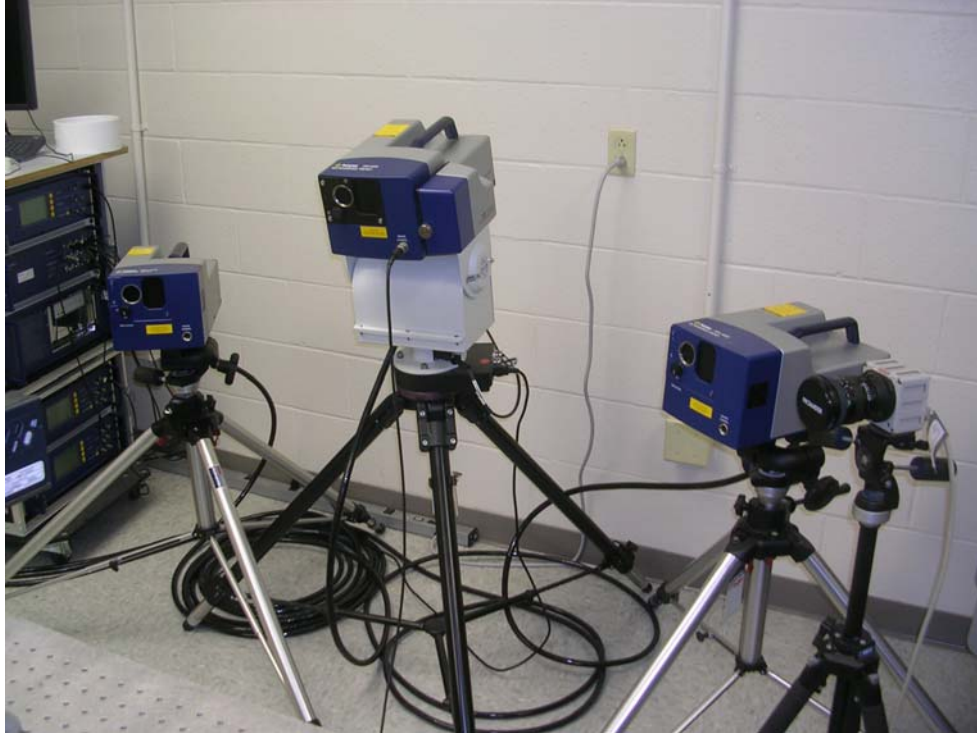
Figure 12: 3-D Laser Vibrometer Setup
