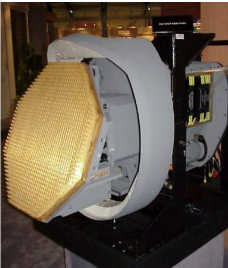
Figure 26. AN/APG-79 AESA Radar 28
