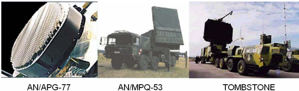
Figure 2. Examples of Radars That Use Irregular Scan Patterns
