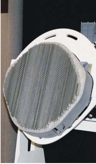
Figure 25. The AESA Antenna Used in the AN/APG-77 Radar 27
