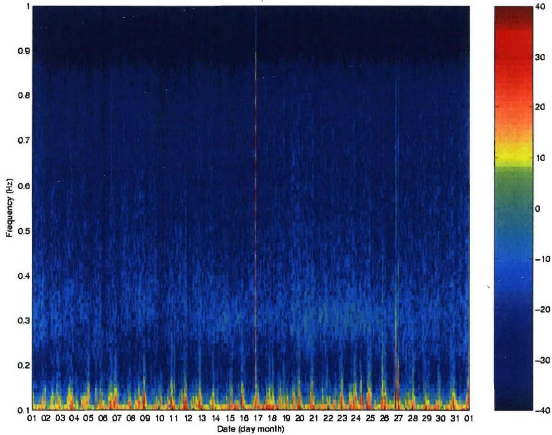
**Figure A-35. Spectrogram for all of 2003 (upper panel) and January 2003 (lower panel) at IS59 in the 0.1-1 Hz frequency band. The upper panel shows the annual variability in the microbarom amplitude and frequency, whereas the lower panel shows the diurnal variability introduced by boundary layer wind fluctuations.**
