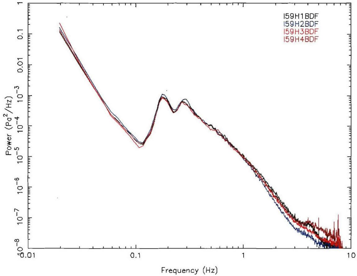
**Figure A-34. Acoustic power spectral density observed at I59US site on June 16, 2003 18Z (8am Local). Colored lines represent power observed by the four components of the infrasonic array.**
