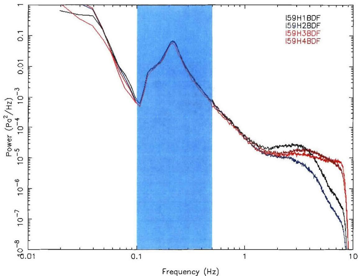
**Figure A-3. Acoustic power spectral density observed at I59US site on January 4, 2003 18Z (8am Local). Colored lines represent power observed by the four components of the infrasonic array. Power (Pa<sup>2</sup>/Hz) is on the vertical axis, acoustic frequency (Hz) is on the horizontal axis. Blue shaded region represents microbarom frequency range. The ~0.2 Hz peak is common throughout the year at I59US, which theoretically corresponds to ocean waves of 10 sec.**
