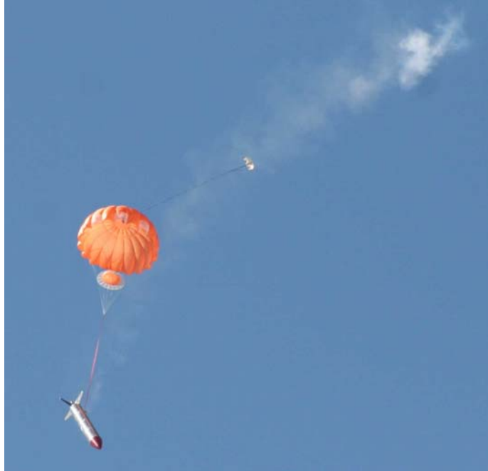
Figure 9. P-7A Parachute Deployment
