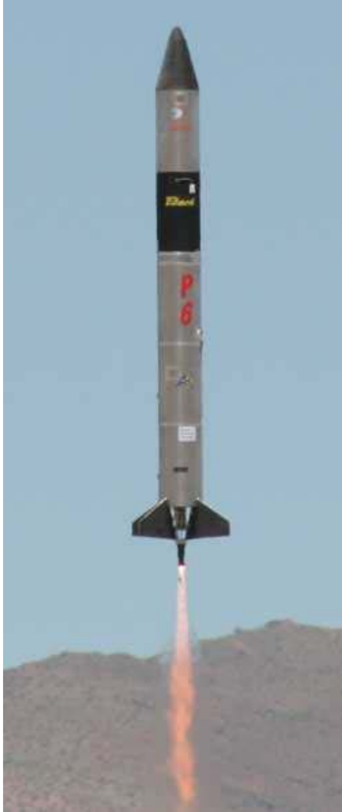
Figure 3. Prospect 6 - Full Scale Prototype NLV in Flight
