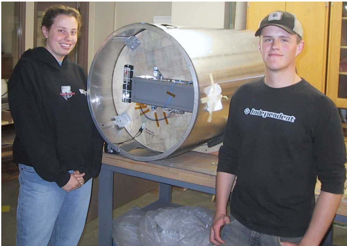
Figure 6. Students with Cal Poly SLO P-POD CubeSat Deployer Mounted in the P-7 Interstage
