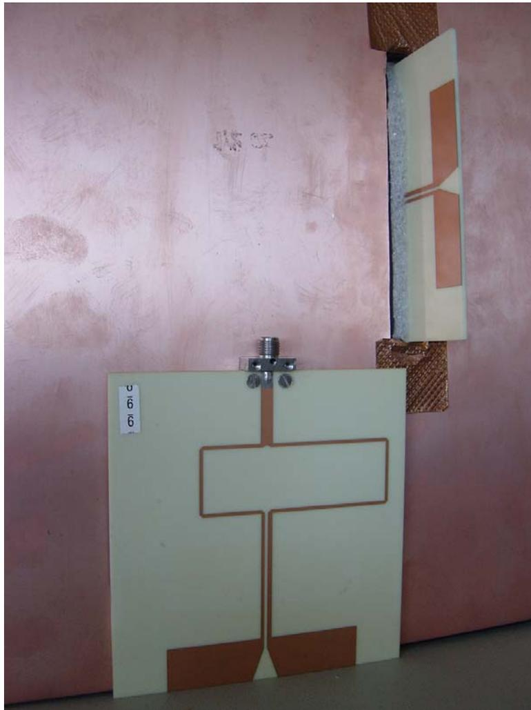
Figure 28. Two dipole elements, of which one is mounted in a ground plane.
