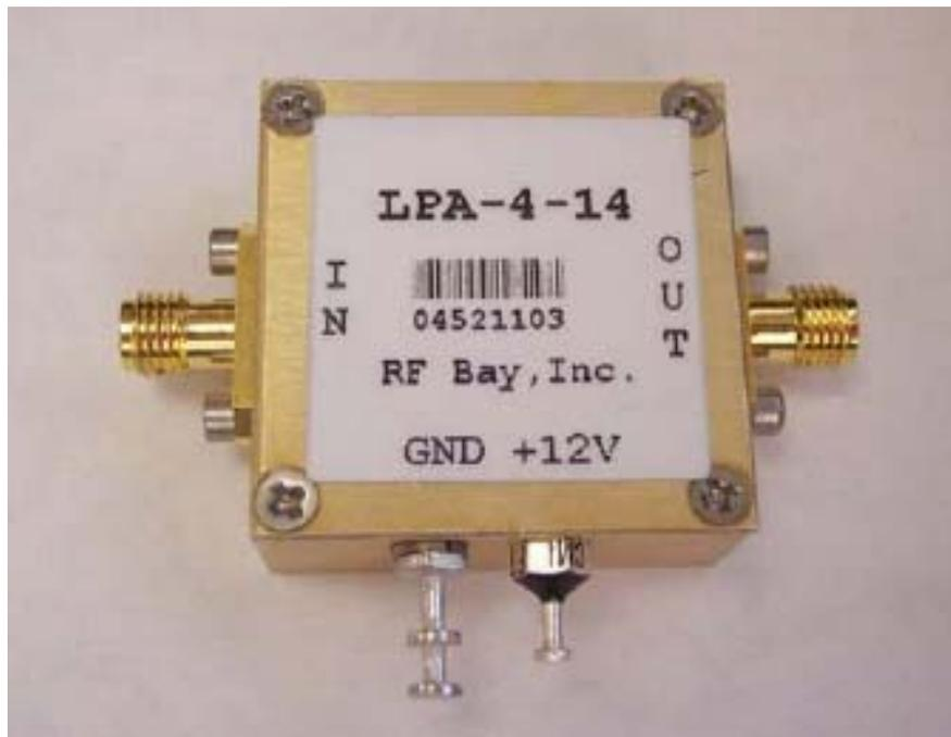
Figure 22. Low-power amplifier LPA-4-14 from RF Bay, Inc.
