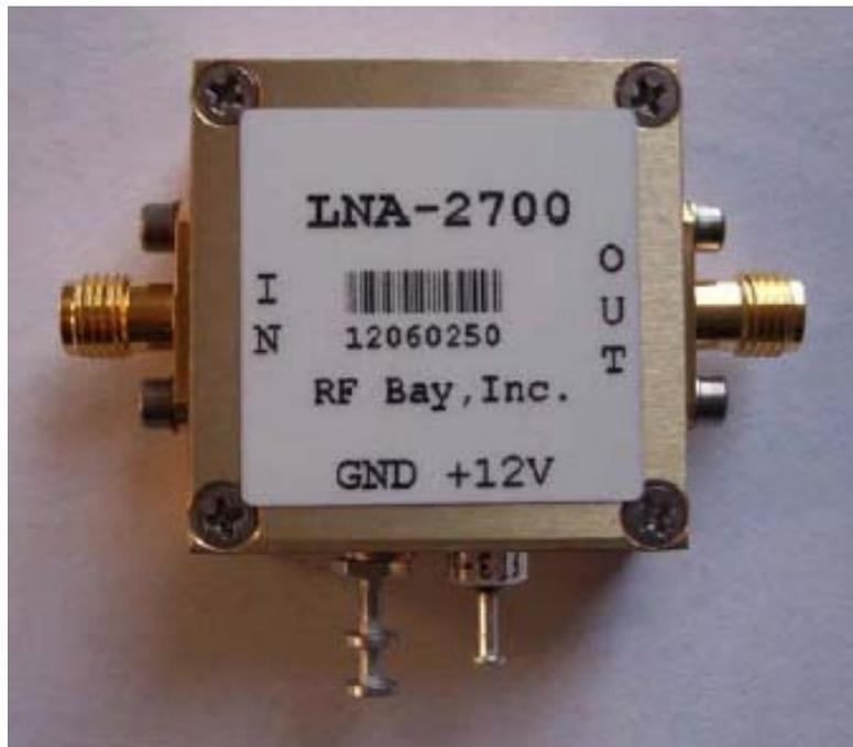
Figure 32. Low-noise amplifier LNA-2700 from RF Bay, Inc.
