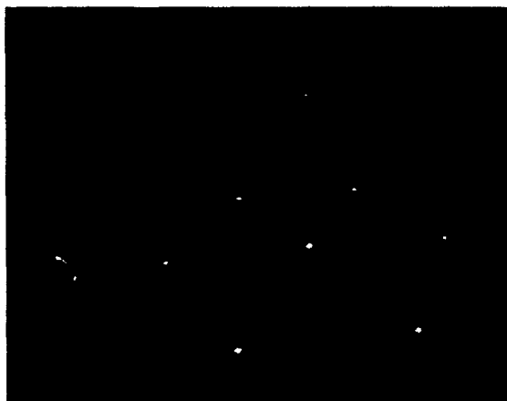
Figure 3. Diffraction of the (111) oriented Inverse opal. Note the six-fold symmetry of the spot pattern.
