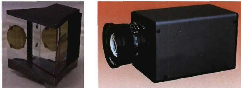
Figure 2.1 Realised prism assembly (left) and the polarisation camera (right).
