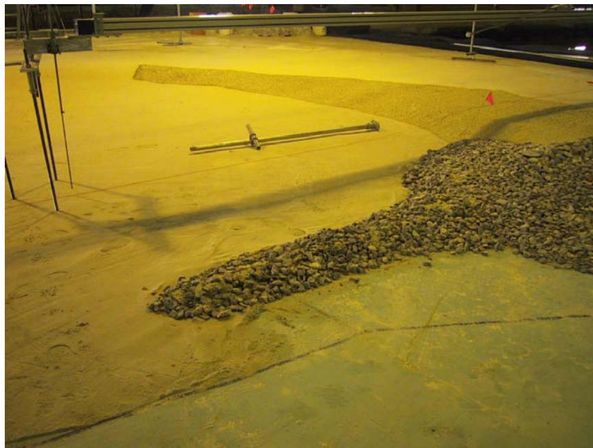
Figure 23. Gravel transition seen from navigation channel.
