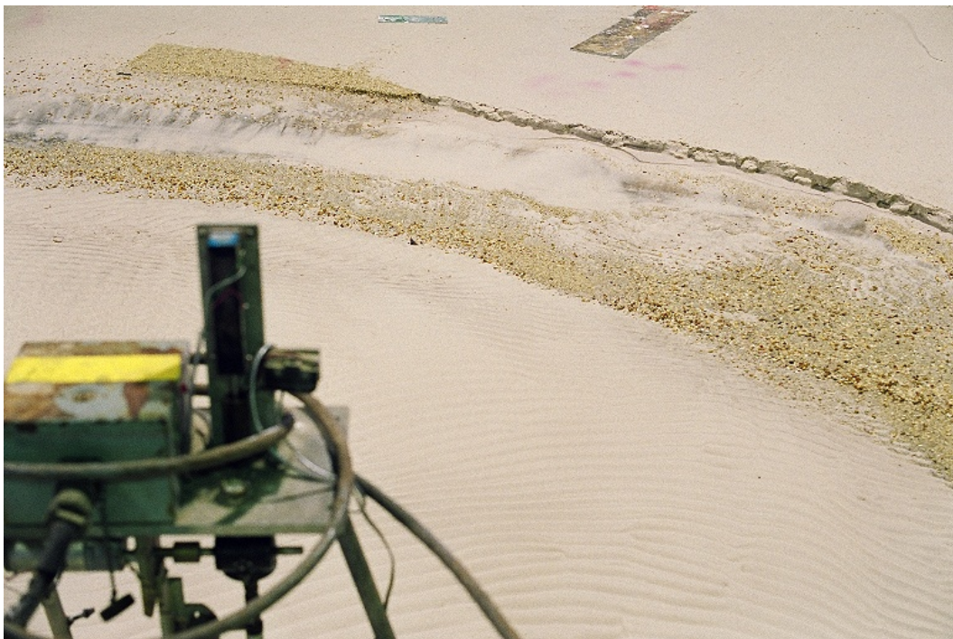
Figure 37. Dune scarp and gravel/cobble removal between profiles P2 and P3 (second calibration experiment).
