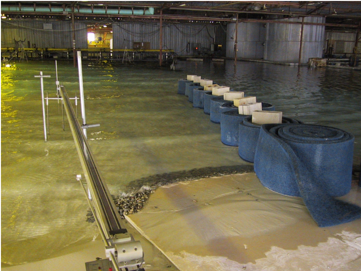
Figure 45. Barrier structure off Point Chehalis used to reduce strong longshore current.
