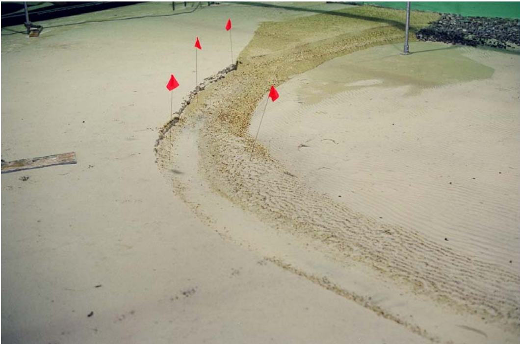
Figure 49. Erosion of gravel transition region.
