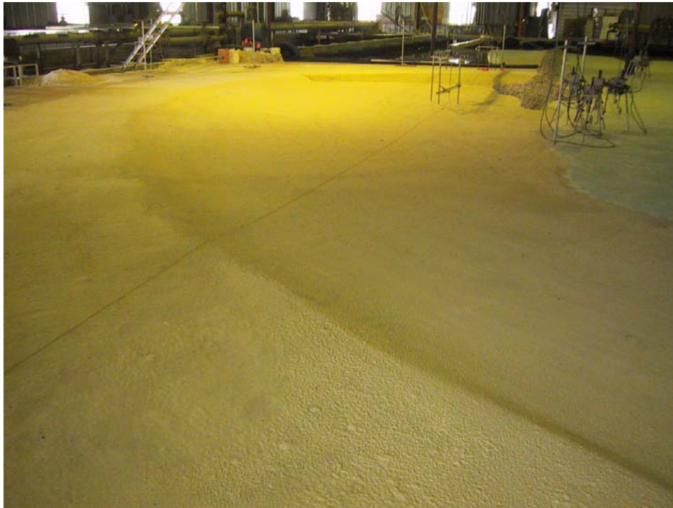
Figure 21. Molded beach looking westward toward south jetty.
