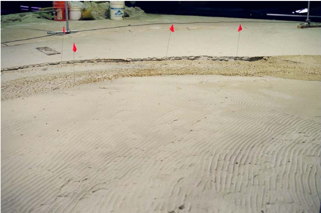
Figure 50. Head-on view of gravel transition erosion.
