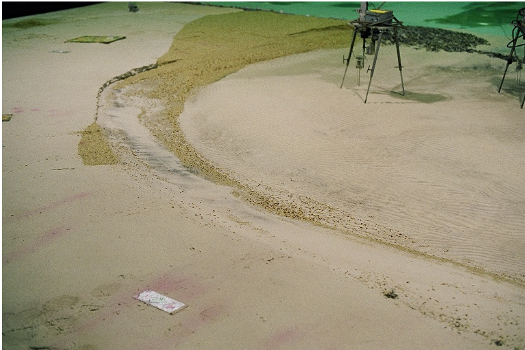
Figure 36. Erosion at western end of Half Moon Bay physical model (second calibration experiment).
