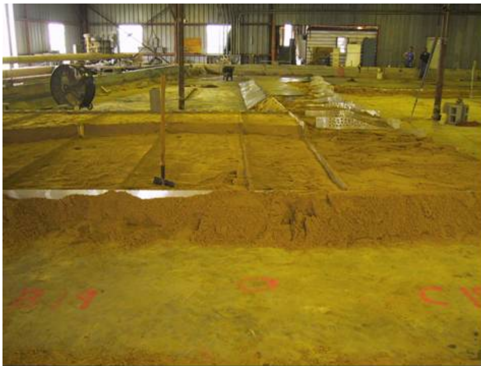
Figure 13. Finishing fixed-bed portion in westward region of Half Moon Bay.
