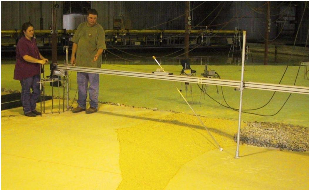
Figure 30. Movable-bed profiler moving over beach near diffraction mound.
