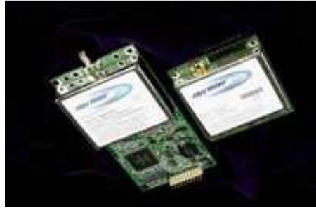
Figure 2.5: Freewave FGR09CS Wireless Modem [4]
