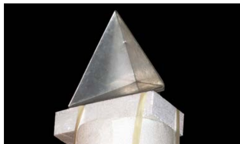
Figure 14: Corner Reflector on Polystyrene Column
