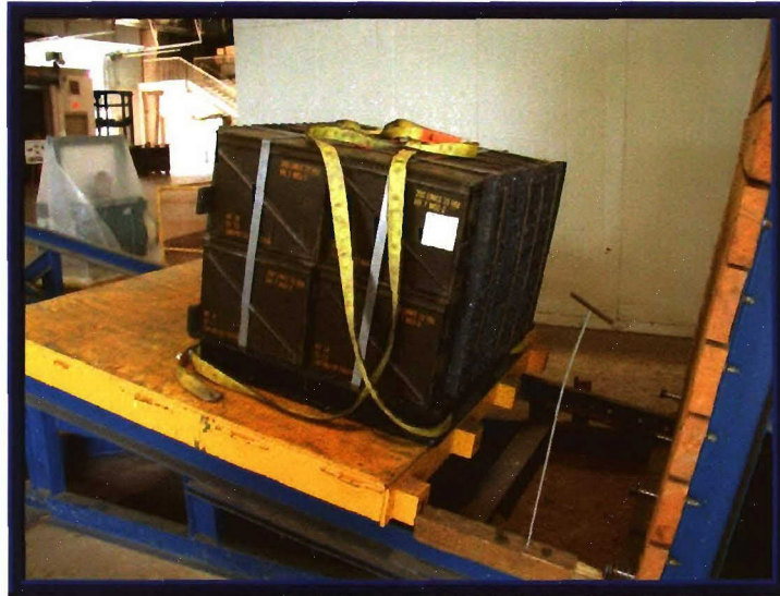
Photo 12. Test Setup for Incline Impact Tests.
