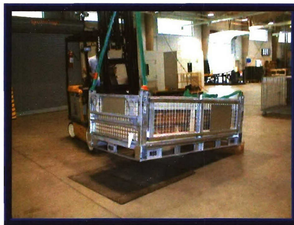
Photo 3. Example of Edgewise-Rotational Drop Test (MSTF Low)
