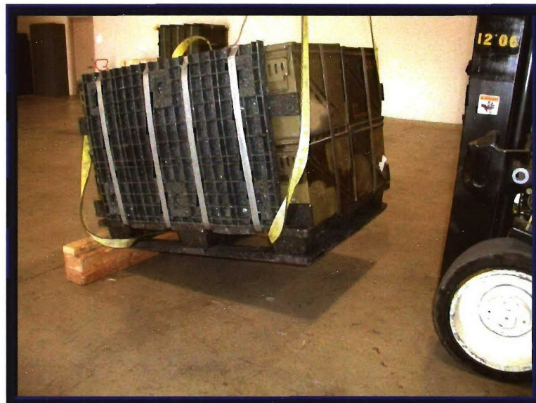
Photo 11. Test Setup for Edgewise Drop Tests.
