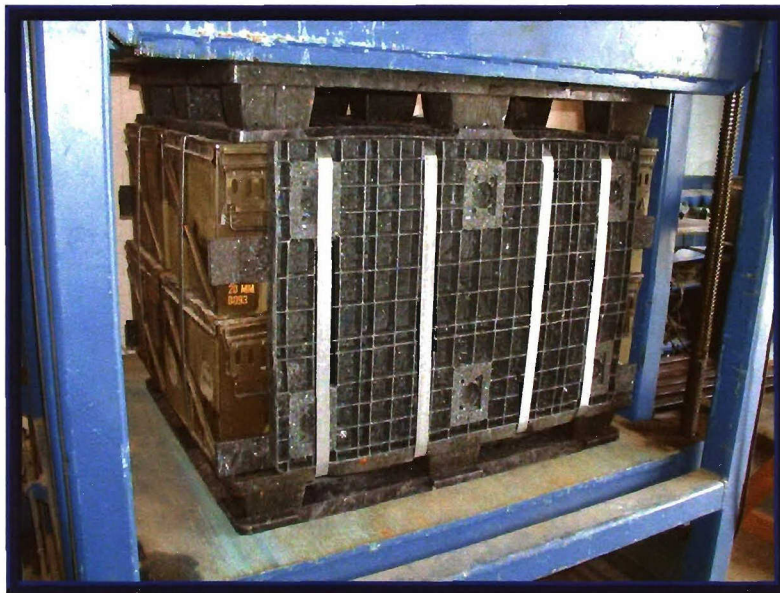
Photo 5. Test Unit in the Stacking Test.
