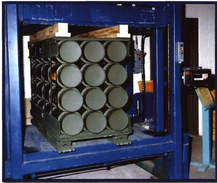
Photo 1. Example of Stacking Test.
