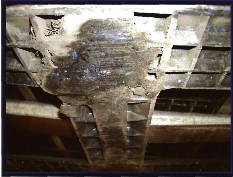
Photo 7. Melted Skid During Repetitive Shock Testing.
