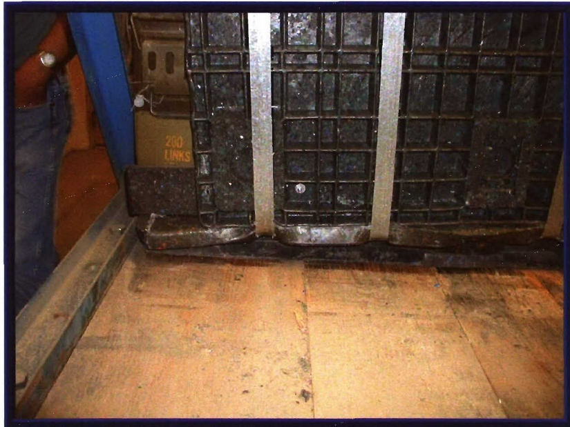
Photo 6. Collapse of Pallet During Repetitive Shock Testing.
