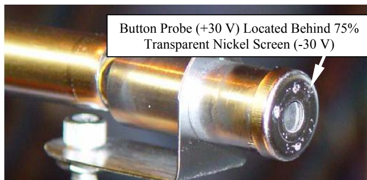
Figure 2. Probe used to measure ion current density profiles.
