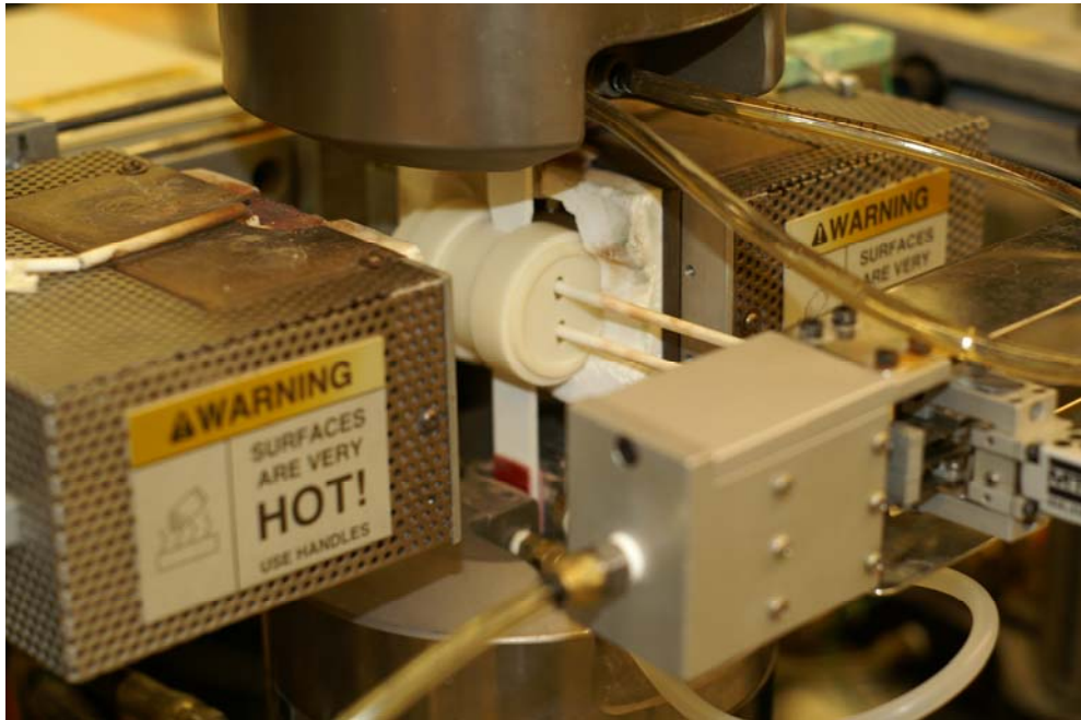
Figure 11. Amteco Hot-Rail Furnace
