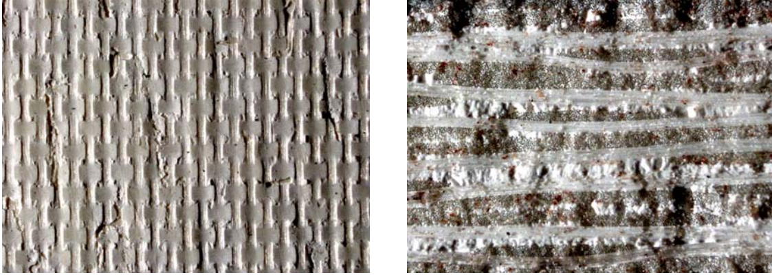
Figure 6. Surface Microstructure of as received Material N720/AS
