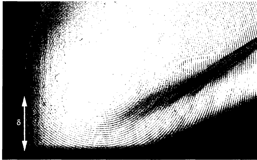
Figure D.2: Schlieren image of STBLI, p_0 = 15psi , BVO
