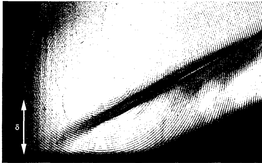
Figure D.6: Schlieren image of STBLI, p_0 = 25psi , BVO
