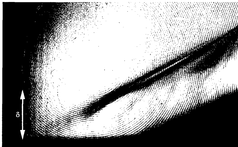
Figure D.5: Schlieren image of STBLI, p_0 = 25psi , BVC
