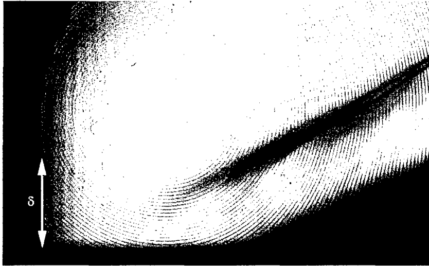
Figure D.1: Schlieren image of STBLI, p_0 = 15psi , BVC
