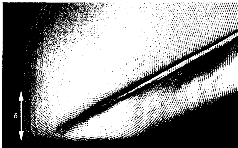
Figure D.7: Schlieren image of STBLI, p_0 = 35psi , BVC
