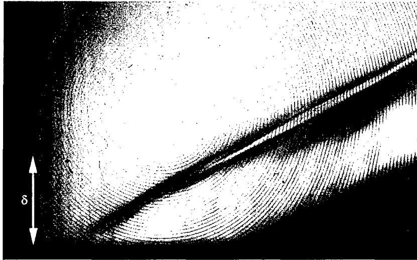
Figure D.8: Schlieren image of STBLI, p_0 = 35psi , BVO
