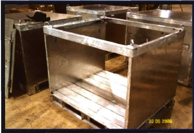
Photo C. Difficult to load due to top frame.
