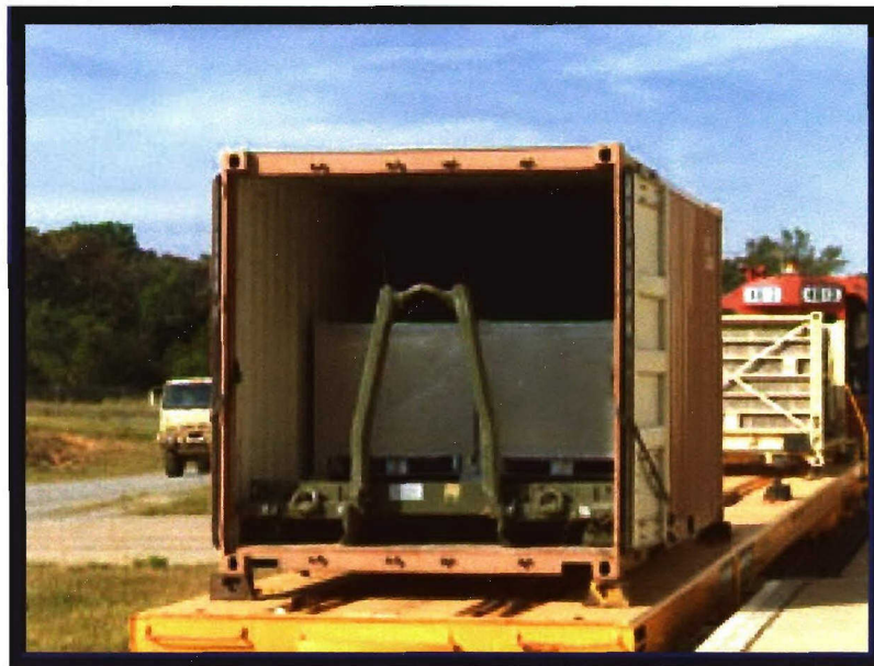
Photo15. Rail Impact Testing of the Navy and BAE JMICs (Prior to Testing)
