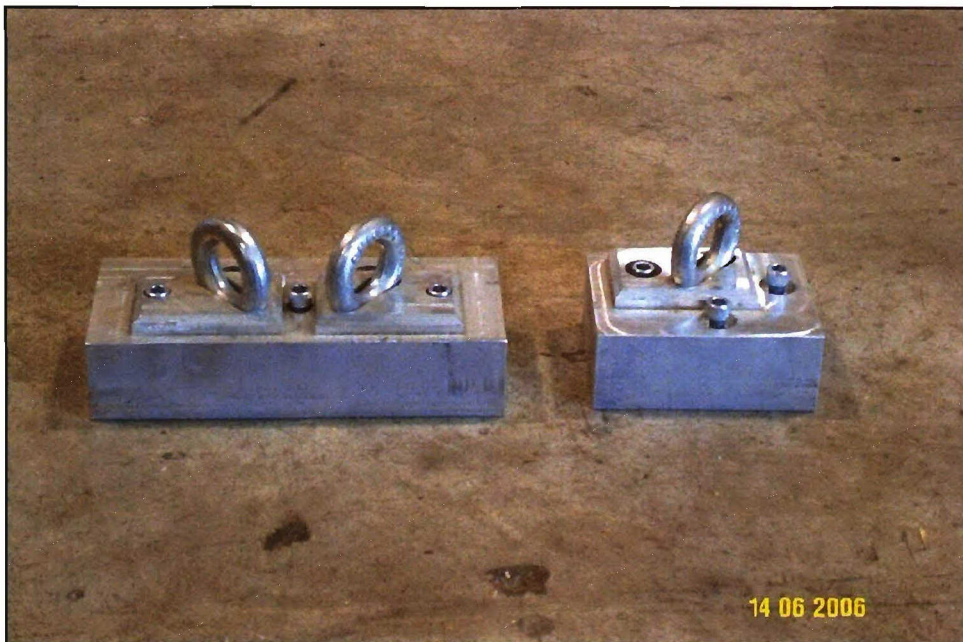
BAE CENTER AND END INTERFACE LOCKS (2 CENTER AND 4 END INTERFACE LOCK REQD PER INTERFACE FRAME)
