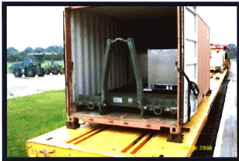
Photo 5. Rail Impact Testing of the BAE JMICs (Prior to Testing)
