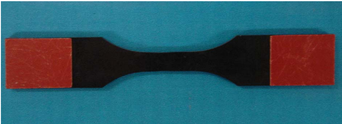
Figure 22: Tabbed PMR-15 Specimen
