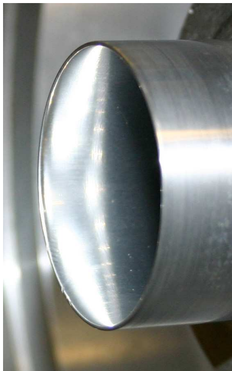
Figure 5.1: Polished surrogate throat with nicks on bleed lip at 7 o'clock
