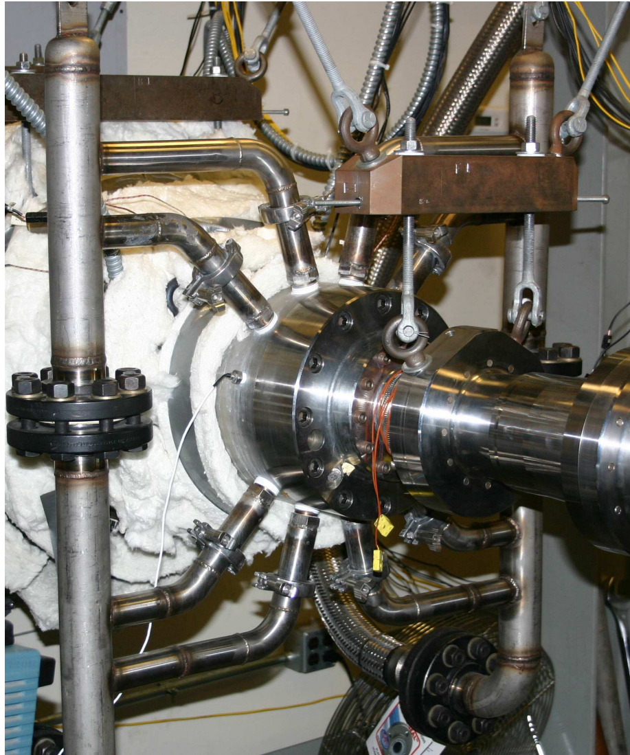
Figure 2.5: Contraction and bleed tubes
