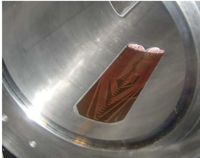
Figure 2.14: Hot-film array installed in Section 8
