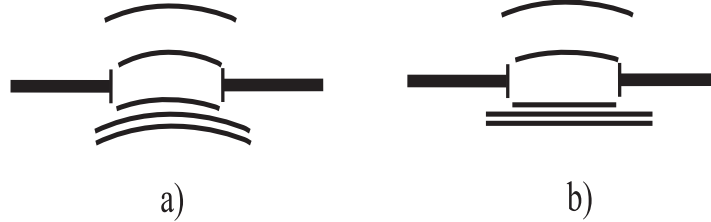
Figure 4: (a) The Fresnel approximation of quadratic phase assumes a spherical wave at the aperture whereas (b) the “more stringent” Fraunhofer criterion assumes a constant phase at the aperture, a more distant and / or smaller image.
