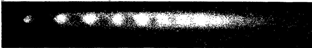
Figure 12 - Flame from 1500-lb-thrust oxygen-alcohol motor
