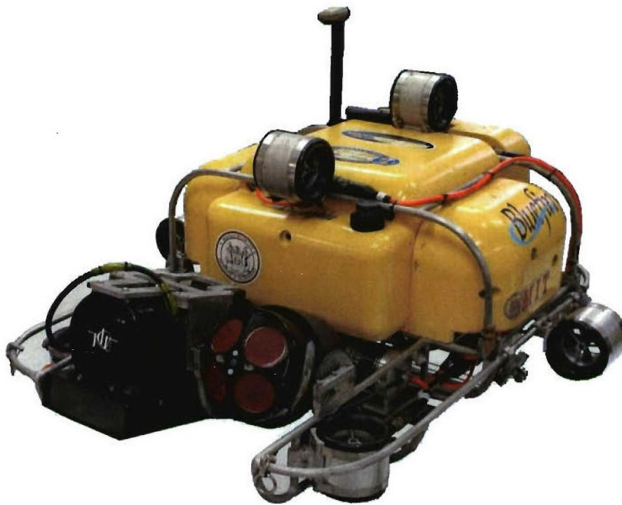
Figure 2. The Bluefin/MIT Hovering Autonomous Underwater Vehicle (HAUV).
