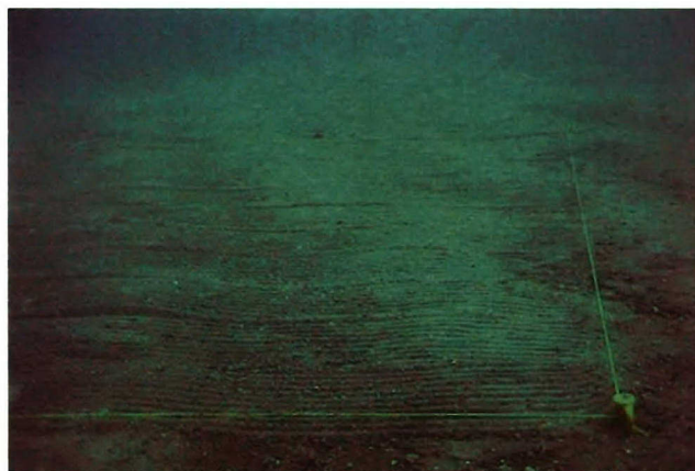
Figure 2. Photograph of the sediment surface raked with a 1.95-cm tine spacing during the SAX99 experiments. The rake had triangular teeth cut at 45° but raking was accomplished with the rake held at an angle roughly 30° to the sediment surface. The resultant ripple amplitude (0.57 cm) was approximately equal to amplitude for a ripple given the measured angle of repose (28°) of the sediment.
