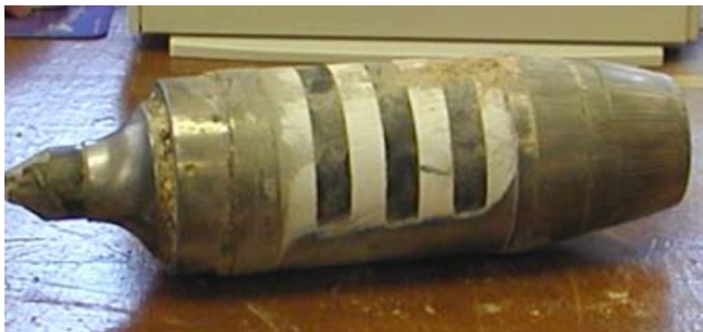
Figure 10. Recovered XM1069 through bunker wall into recovery array.
