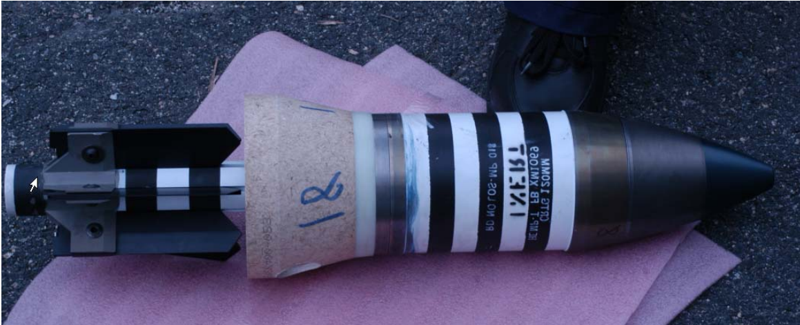
Figure 9. Pre-assembly photograph of the XM1069 with cartridge case adapter.
